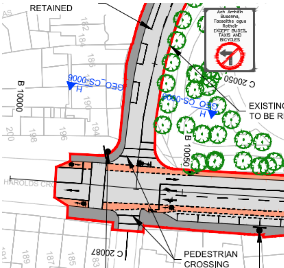
Image 4.12: Preliminary Design of the Proposed Scheme Tie-in with the Templeogue / Rathfarnham to City Centre Core Bus Corridor Scheme at Harold's Cross Road and Parkview Avenue Junction
